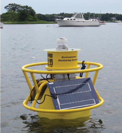
The EMM68 buoy is lightweight and easy to deploy from shore or small boat
